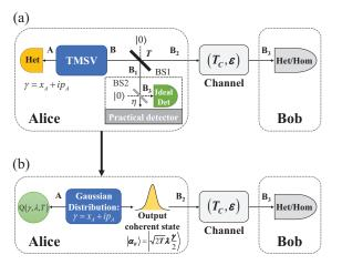
FIG. 1: (color online)(a) Entanglement-based (EB) scheme of CV QKD with photon subtraction. (b) Prepare-and-measure (PM) scheme of CV QKD with *virtual* photon subtraction. Other notations: Het: heterodyne detection. Hom: homodyne detection. BS1(2): beamsplitter.  $\gamma$ : Alice's measurement result.  $\lambda$ : parameter of TMSV.  $Q(\gamma, \lambda, T)$ : postselection filter function.  $T(\eta)$ : transmittance of BS1(2).  $T_C, \varepsilon$ : channel parameters
